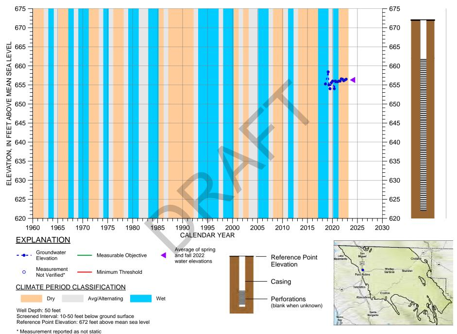
HYDROGRAPH OF MEASURED GROUNDWATER ELEVATION FOR 18MW-0191
