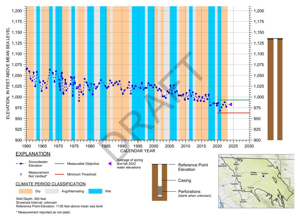
HYDROGRAPH OF MEASURED GROUNDWATER ELEVATION FOR 26S/15E-29N01
