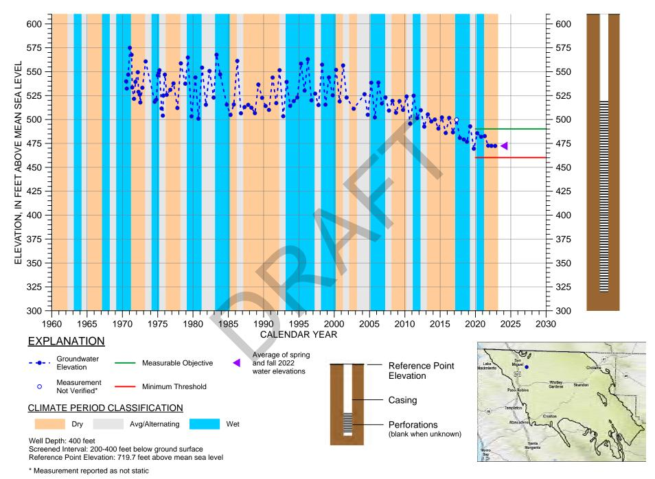
HYDROGRAPH OF MEASURED GROUNDWATER ELEVATION FOR 25S/12E-26L01
