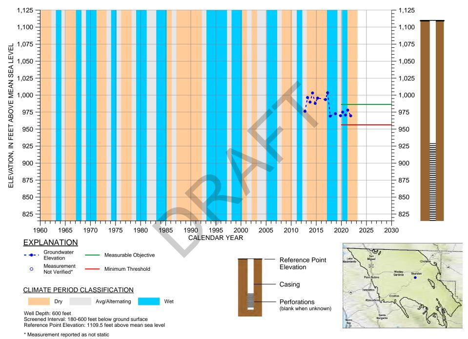
HYDROGRAPH OF MEASURED GROUNDWATER ELEVATION FOR 26S/15E-29R01
