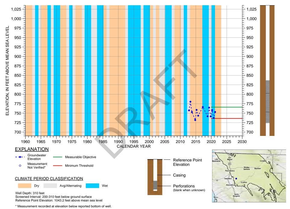
HYDROGRAPH OF MEASURED GROUNDWATER ELEVATION FOR 27S/13E-30F01
