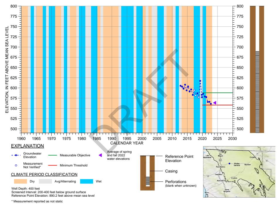
HYDROGRAPH OF MEASURED GROUNDWATER ELEVATION FOR 26S/13E-16N01
