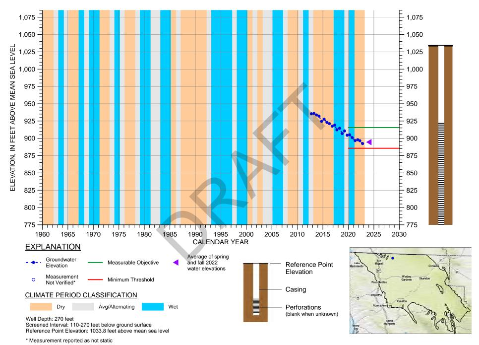
HYDROGRAPH OF MEASURED GROUNDWATER ELEVATION FOR 25S/13E-08L02
